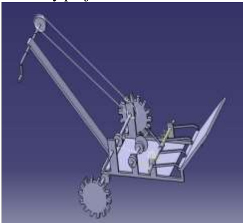
Fig 3.1: Design of rice planting type machine in CATIA
